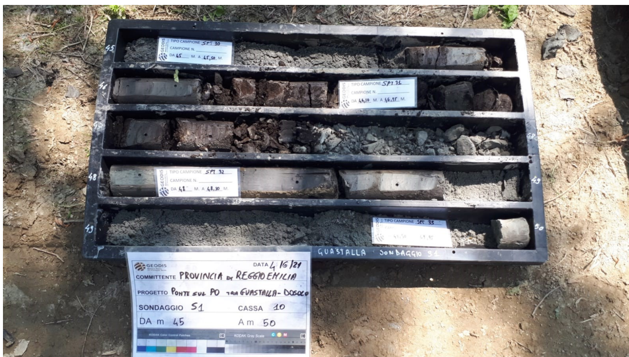
Fig. 15 - Sondaggio S1 cassa 10 (45,00-50,00m)
