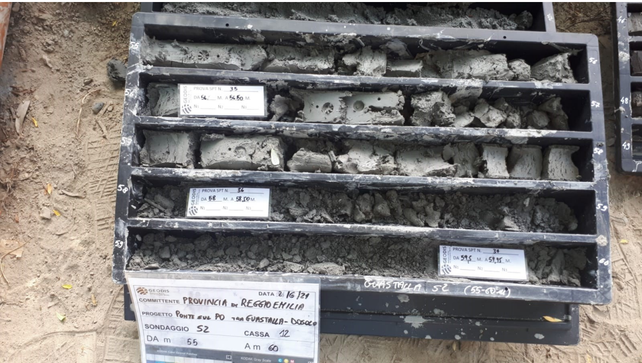
Fig. 30- Sondaggio S2 cassa 12 (55,00-60,00m)
