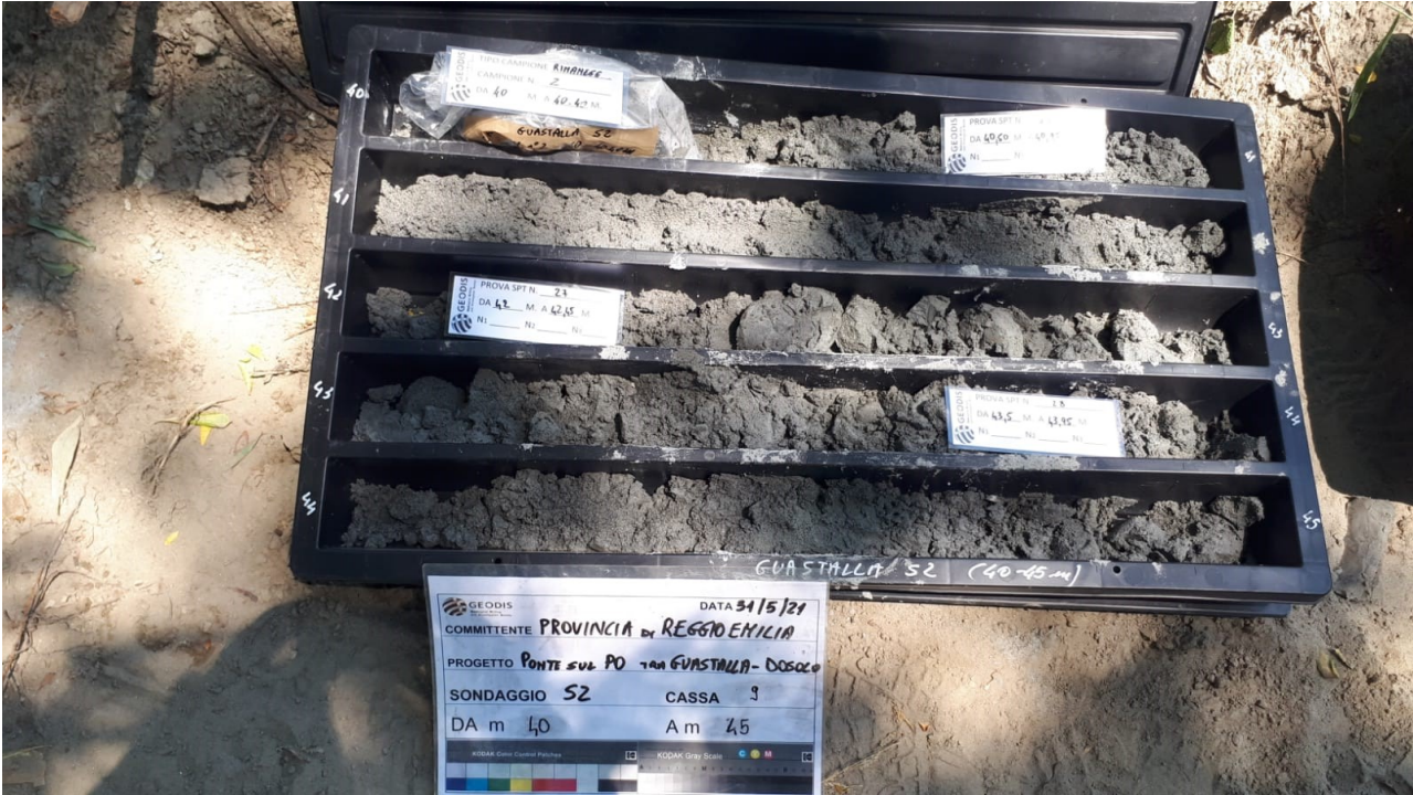
Fig. 27 - Sondaggio S2 cassa 9 (40,00-45,00m)
