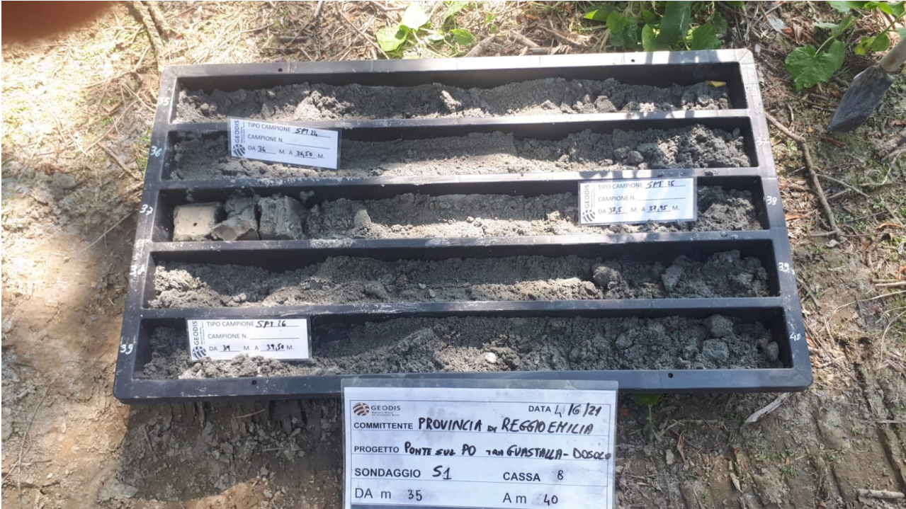
Fig. 13 - Sondaggio S1 cassa 8 (35,00-40,00m)
