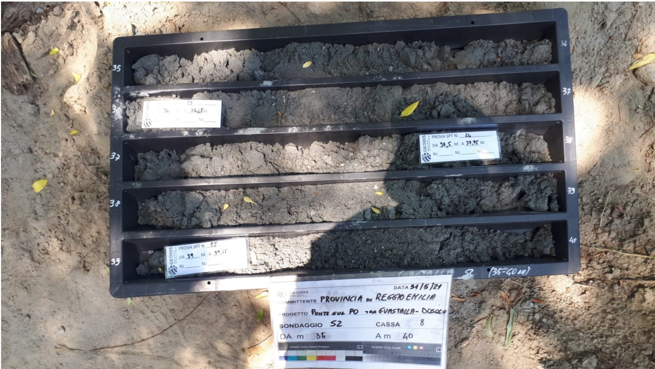
Fig. 26- Sondaggio S2 cassa 8 (35,00-40,00m)
