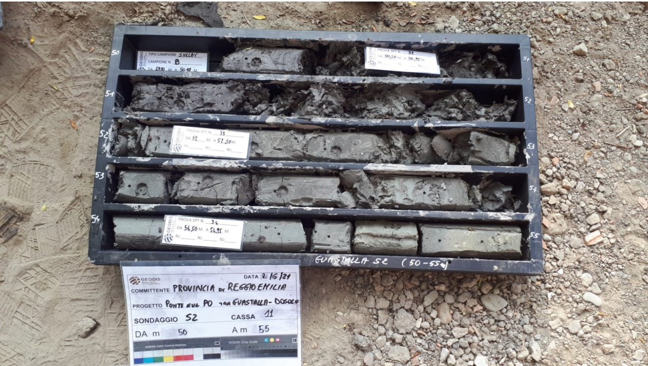
Fig. 29 - Sondaggio S2 cassa 11 (50,00-55,00m)
