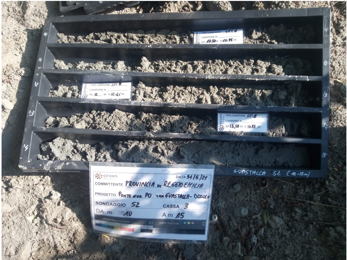
Fig. 21 - Sondaggio S2 cassa 3 (10,00-15,00m)
