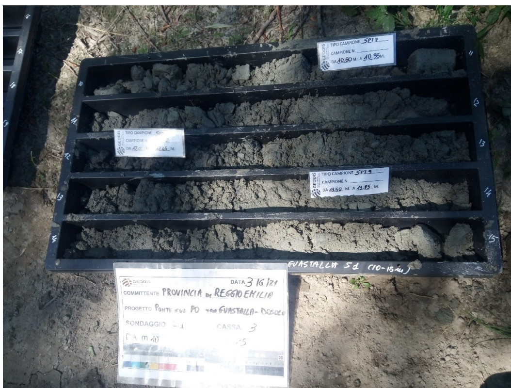
Fig. 8 - Sondaggio S1 cassa 3 (10,00-15,00m)
