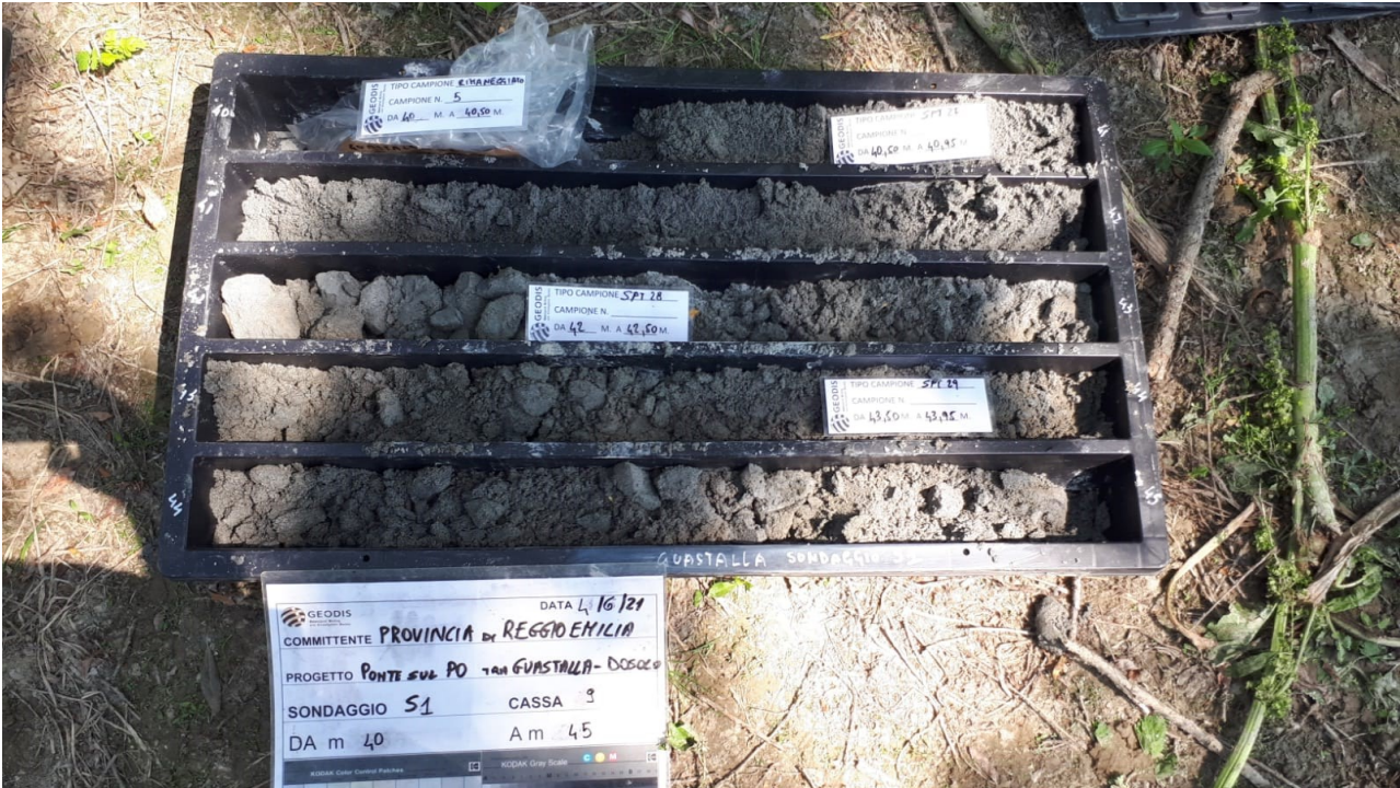
Fig. 14 - Sondaggio S1 cassa 9 (40,00-45,00m)
