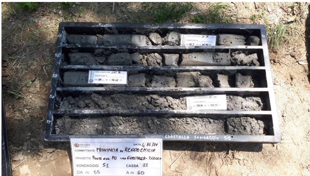
Fig. 17 - Sondaggio S1 cassa 12 (55,00-60,00m)
