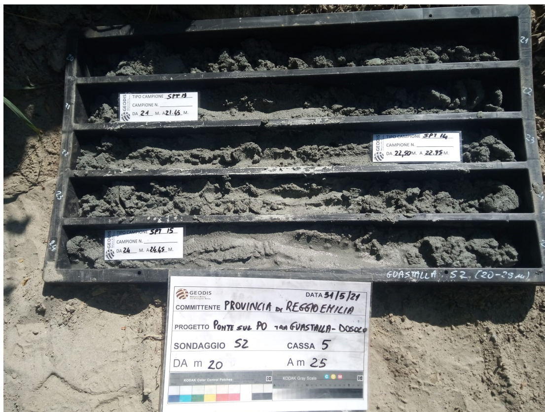
Fig. 23 - Sondaggio S2 cassa 5 (20,00-25,00m)
