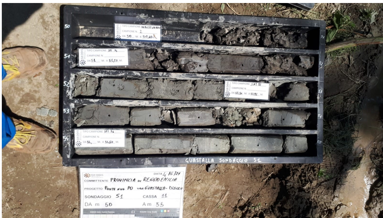
Fig. 16 - Sondaggio S1 cassa 11 (50,00-55,00m)
